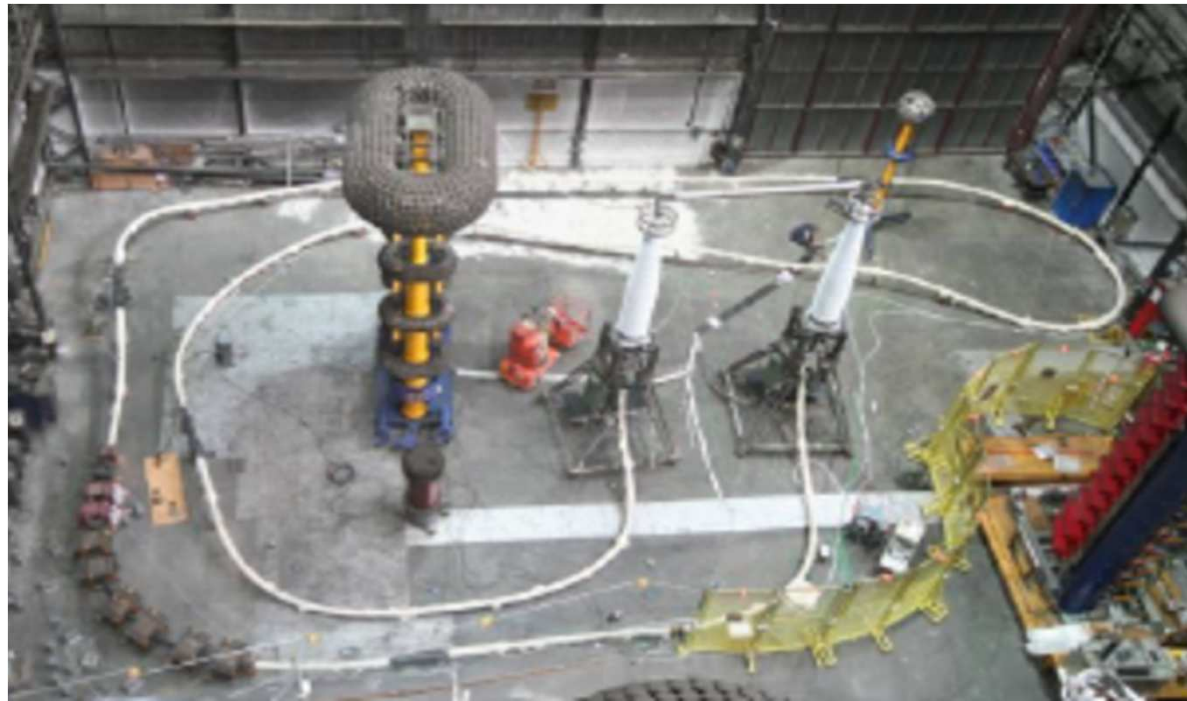
HVDC cable system during a Prequalification Test according to CIGRE TB 496
